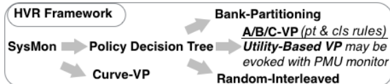
Figure 12. HVR Framework in a nutshell (with Curve-VP). Note that Curve-VP can be replaced by bank partitioning and Random-Interleaved policies.
